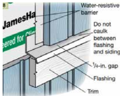
Figure 8: Correct Flashing Installation
