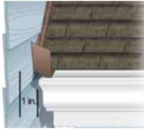
Figure 3: Proper Kick-Out Flashing
